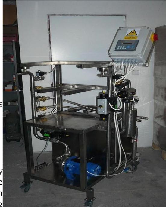
All liquid flows are monitored by individual conductivity probes. Washes are pulsed for optimum cleaning.
